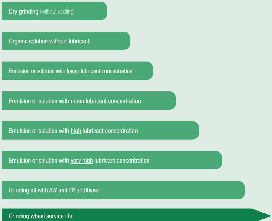
Relative service life of the grinding wheel depending on the cooling lubricant used
