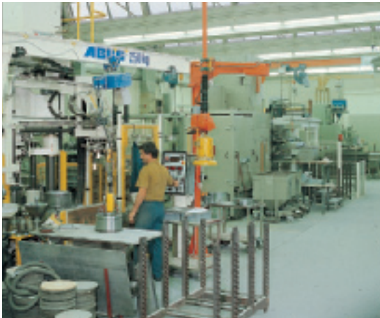
NC-controlled presses ensure the exact duplication of the homogenous wheel structure.
