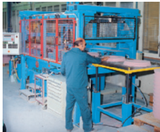
Winterthur grinding wheels are checked for imbalance in a single operation on a computer controlled machine.
